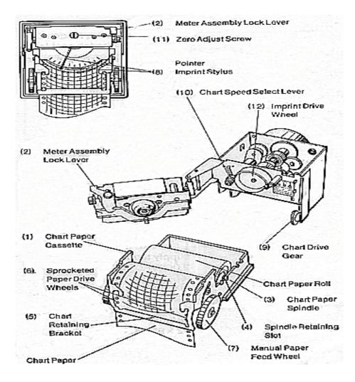
Note that the stylus may not move freely if the recorder is in the imprint section of its operating cycle with the stylus pressed against the chart paper. In this case the recorder chart motor should be operated for a few seconds until the imprint pressure is released, or the imprint drive wheel (12) can be manually rotated. The chart paper can be manually advanced by operating the manual paper feeding wheel (7) to set the desired zero time position.
