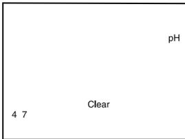
1. Press **Setup** once to clear all buffers you have entered. If you are sure you want to clear the buffers, press **Enter**. The meter clears all buffers and returns to **Measuring**.
