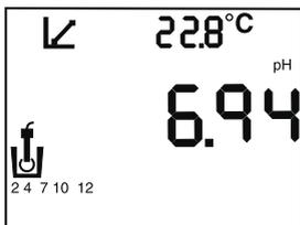
4. Press **Standardize**. The meter recognizes the buffer and flashes a buffer icon. When the signal is stable, the buffer is entered. By pressing **ENTER** you can also enter the current buffer directly.
