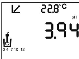
6. To enter a second buffer, place the electrode in the second buffer solution, stir, allow time for the electrode to stabilize, and press **Standardize** again. The meter recognizes the buffer and displays the first and second buffer values.
