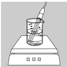
11. Standardize your pH meter using at least two buffers with pH values bracketing the expected pH of your samples. Stirring with a magnetic stir bar provides faster electrode response.
