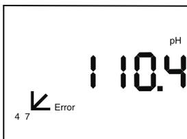
2. The meter will display **Error** when it detects an error in electrode response. During standardization, the message indicates that the electrode is less than 90% or more than 105% of the correct response. The **Error** message can indicate either a bad electrode or bad buffer(s).
