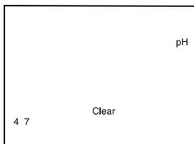
3. Clear existing buffers when doing a new 2- or 3-point standardization. Use the **Setup** button. Also use the **Setup** button to select the individual sets of buffers. (See page 13.)
