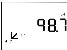
7. Next, the meter performs a diagnostic test of the electrode. The display indicates either Good Electrode ("OK") or Electrode Error ("Error"). The meter also displays the slope of the electrode.
