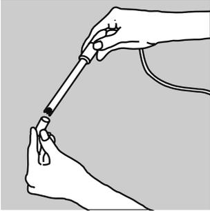
2. Before first use of your electrode, or whenever the electrode is dry, soak overnight in a standard solution or KCl solution.
