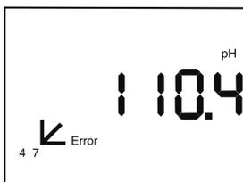
8. **Error** indicates that your electrode or the buffer is not working properly, or a wrong set of buffers has been selected. The electrode response must be between 90 and 105% slope. (See Troubleshooting, on page 21.) Press **Enter** to clear the Error, then try re-entering the buffer as described in step 6.
