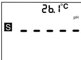
1. If the signal from the electrode is out of range, the display will show “—”. This may happen when the electrode is not immersed in a solution.
