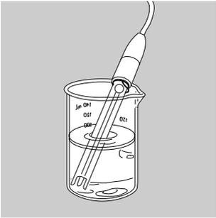
3. Remove the shorting cap on the pH meter connector. Install the electrode by plugging the BNC and ATC connectors into the jacks on the rear panel.
