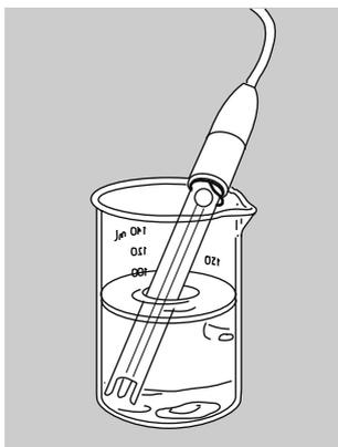
1. Immerse electrode in a standard solution.
