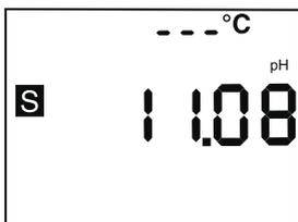
3. If the meter detects an error in the temperature measurement, the display shows “—°C.” If you do not use a temperature probe, the meter uses the standard temperature (25°C).
