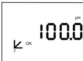
5. The meter displays the slope of the electrode as 100.0%. On entering a second or third buffer, the meter performs a diagnostic check on the electrode and displays the slope. (See step 7 ff.)
