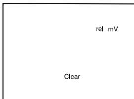
5. To clear an mV offset and return to absolute millivolt mode, press **Setup**. The meter displays a flashing Clear icon, and shows the current relative millivolt offset.
