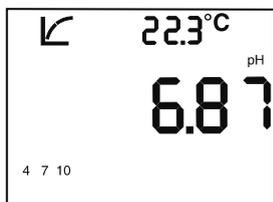
10. After entering three buffers, the **Standardizing** icon goes out and the **Measuring** icon appears on the display to indicate that the meter returns to **Measuring** operation.
