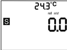
4. When the signal becomes stable, or when you press **Enter**, the current absolute mV value (offset) becomes zero relative millivolts.
