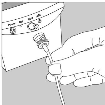
4. To test the pH electrode, place it in a good pH 7 buffer. Press **pH/mV** to use the mV mode, and note the millivolt reading. Repeat for either a pH 4 or pH 10 buffer. The electrode signals must be within the limits shown below (when temperature is approx. 25°C).
