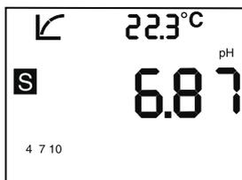
1. Immerse electrode in a buffer solution. Stir gently. Allow the electrode to reach a stable value.
