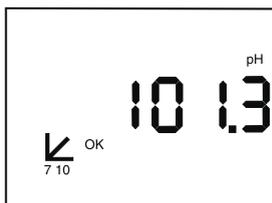
9. To set a third standard, place the electrode in the third buffer solution, stir, allow to stabilize, and press **Standardize**. The results will be the same as in steps 6 and 7, except the display will show three buffer values.
