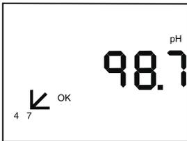
2. Press **Setup** again to show electrode performance, slope and the first and second calibration points. The two buffer values will also be displayed.
