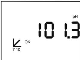
3. Pressing **Setup** again shows the electrode slope between the second and third buffers (if three buffers have been entered) and shows the second and third buffer icons.
